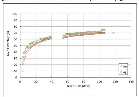
Figure 13-4: Otis Gold Column Leach Tests - Composite MAS-1, P<sub>80</sub> at ½-Inch
