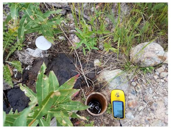
Photo 12-2: Closely Spaced, Variably Marked Drill Hole Collars
