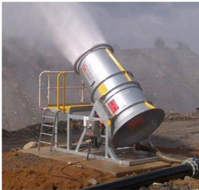
Figure 25-18: Evaporator to Manage HLF Drain-Down
